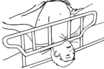
Entrapment under the bed rail
