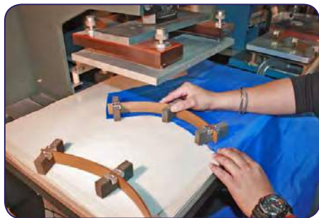
Custom fitting the RF sealing welds.
