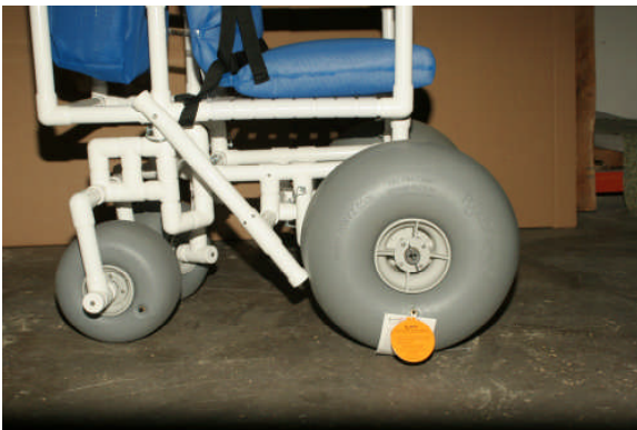
PHOTO 7: PARKING BRAKE ENGAGED
